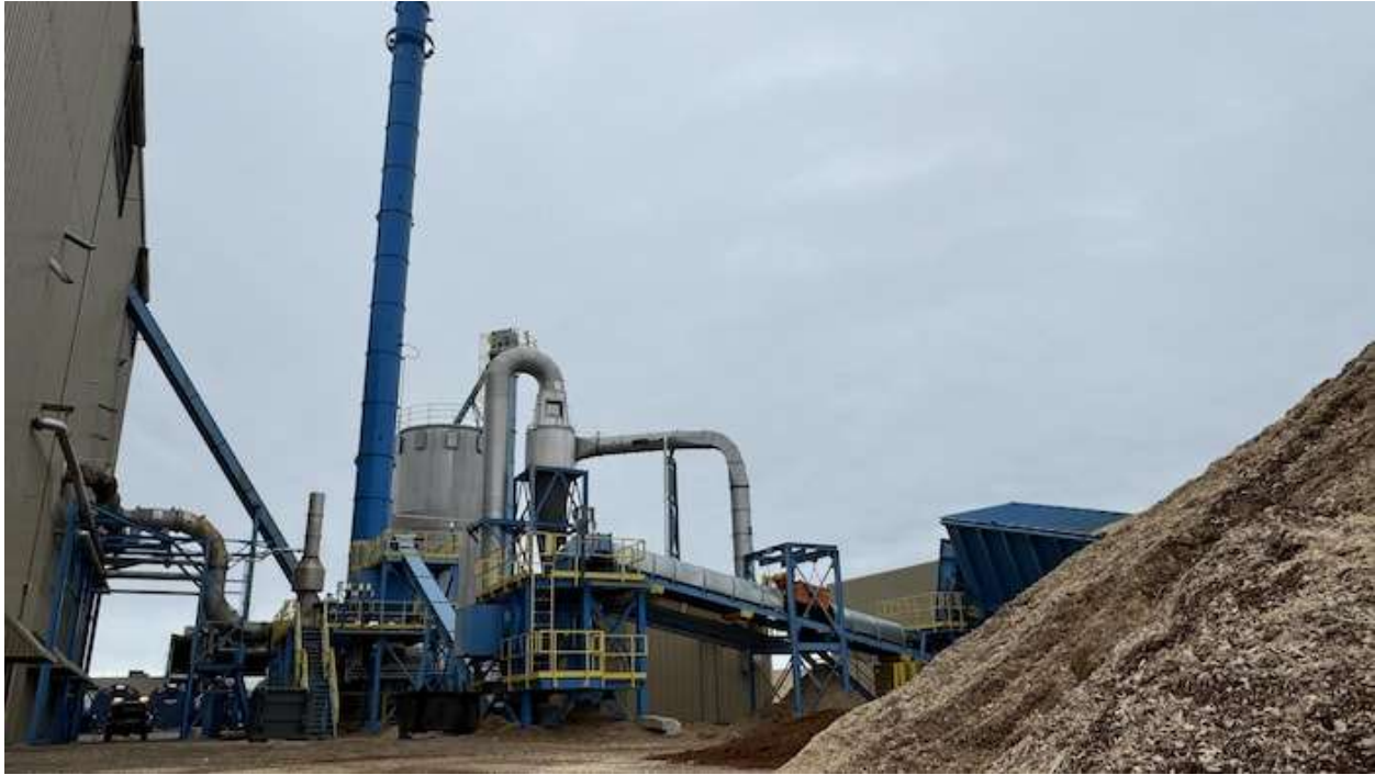
Outside the AE Bioenergy plant, mountains of wood waste are piled up. They will be ground and dried before being transformed into pyrolytic oil. PHOTO: RADIO-CANADA / RENAUD CHICOINE-MCKENZIE
