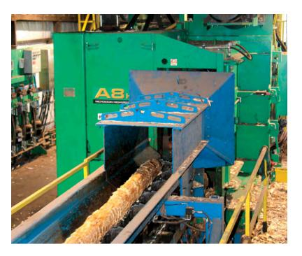
Sawmill updates in 2023 included a screw infeed from Austria-based Springer, and a new Nicholson A8 debarker, which works alongside an older Carbotech double rotor debarker.
