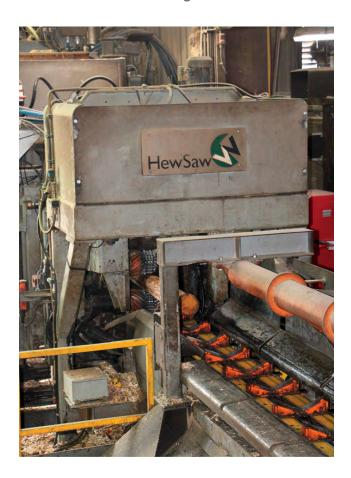
was installed in 2020. Logs greater than five-inch diameter are directed to two bins dedicated to the HewSaw R200 1.1, and smaller logs are sorted to four bins according to diameter class, which feed the HewSaw R200 A.1.
